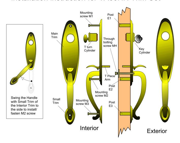
Upon the installation of the Mortise lock case from the Door Edge ,,,,,,...
